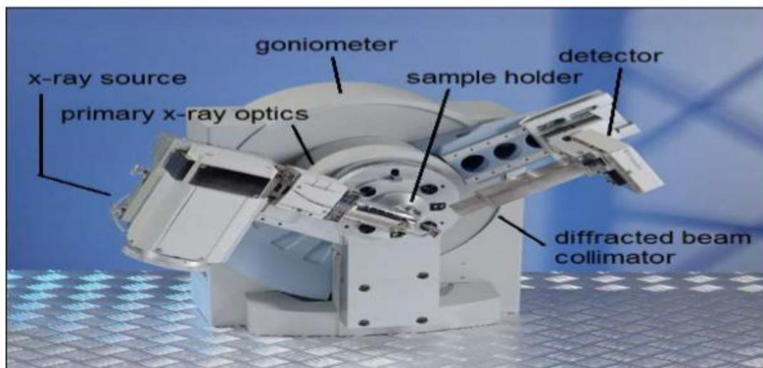
**X-ray Tube:** the source of X-rays
